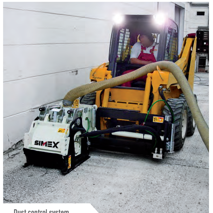
Dust control system
