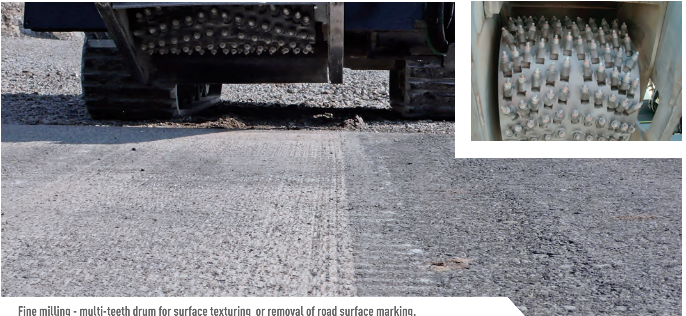
Fine milling - multi-teeth drum for surface texturing or removal of road surface marking.
